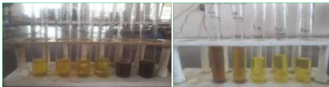
Fig.-1: 1-(5'-Formyl-2'-hydroxy-3'-methoxyphenyl)-3-(substituted phenyl) propane-1,3-diones Compounds 4(a-e) Before Centrifugation
