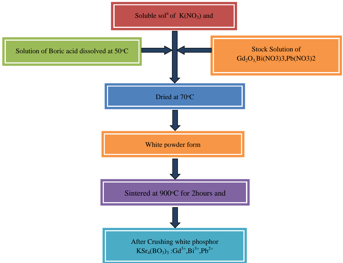
Figure1. -Flowchart of synthesis of phosphors by re crystallization method
